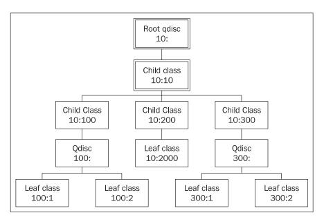
So, basically CBQ or HTB qdiscs allow us to create child CBQ or HTB classes, which we can set up to shape some kind of data. For each child class, we can attach a qdisc for scheduling packets within that child class. Next, we can create leaf classes, which are child classes of the qdiscs we attached to the child classes, or we can create leaf classes as child classes' child classes attached to the root qdisc.
